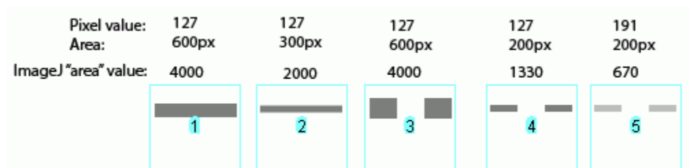
Figure 27. ImageJ deals with gaps in bands just fine. Note however that the "area" values returned by ImageJ are different compared to Figure 26 and Figure 27, because the number of lanes, size of the bands, and density of the bands has changed.
